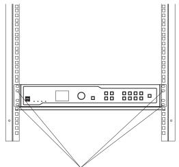
Attach the floating nuts to the bars with square holes, and then fix the device to the bars with screws
